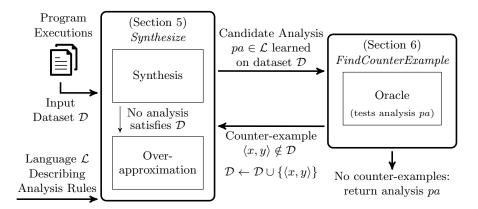
Fig. 1. Overview of our approach to learning static analysis rules from data consisting of three components – a language  $\mathcal{L}$  for describing the rules, a learning algorithm and an oracle – that interact in a counter-example based refinement loop.
